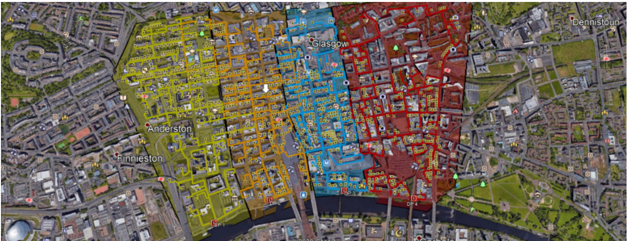
Figure 4. Glasgow city centre divided into four parts - each heated by its own heat pump-iteration 2
